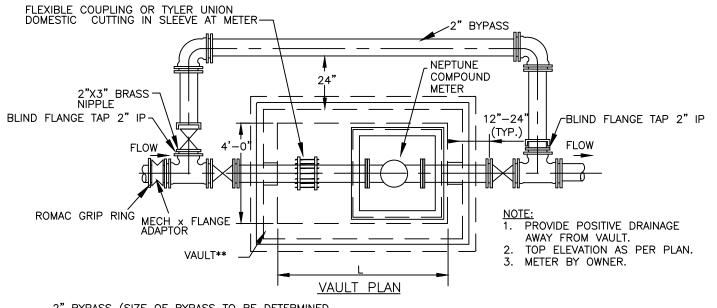
2" BYPASS (SIZE OF BYPASS TO BE DETERMINED BY ENGINEER).
